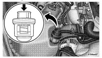
The clear plastic housing on the Filter Minder™ allows you to view the amount of air pressure drop across the filter element. It consists of a diaphragm and a calibrated spring sealed inside the plastic housing. As the air cleaner filter becomes clogged and air pressure drop across the filter element increases, a yellow disc travels along a graduated scale on the side of the Filter Minder<sup>TM</sup>.
